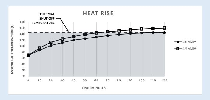
The lower curve of the Heat Rise graph plots the highest current where this pump model can run without a cooling requirement. The upper curve represents the highest current draw of this pump model, under which the thermal breaker would open after approximately sixty (60) minutes and the motor would require approximately thirty (30) minutes of cooling before it restarts. Power cycling should be limited to six (6) times per minute.
